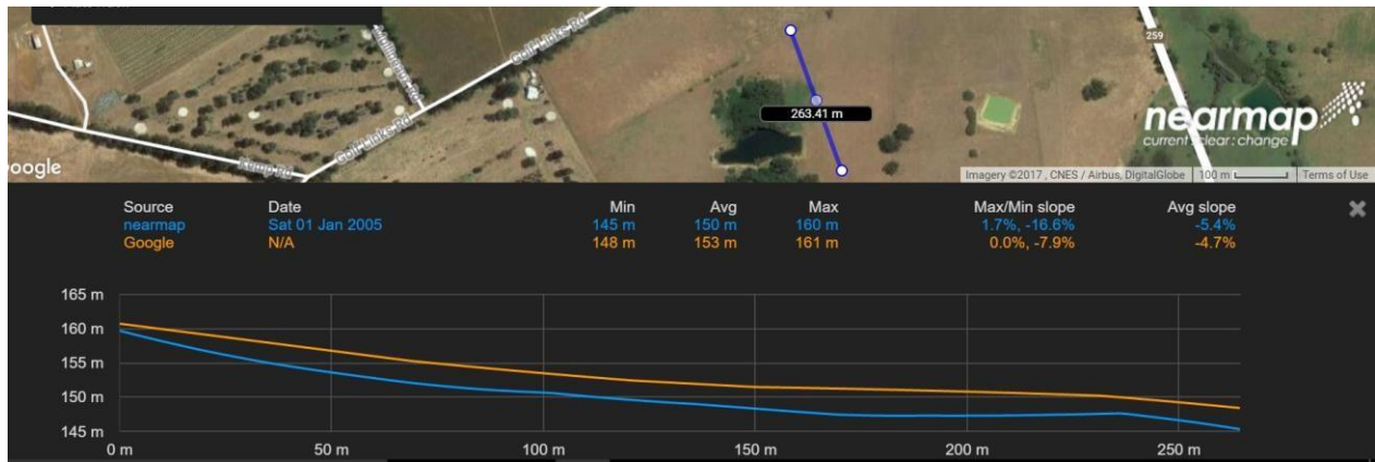
Figure 5. Slope across the lot and neighbouring property to the south of 4.7% (0.4°).
