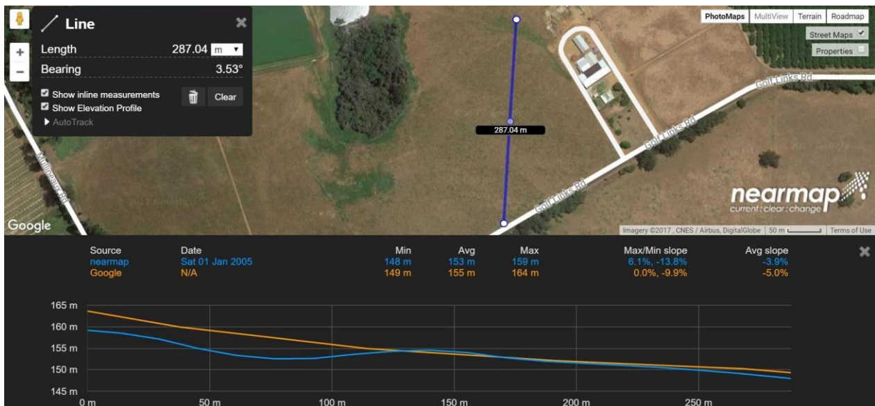
Figure 3. Slope across the neighbouring properties to the north of 5% (0.0.6°).
